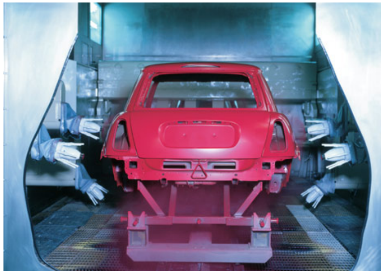
Figure 5. Automated spray painting of a car body in a BMW plant
