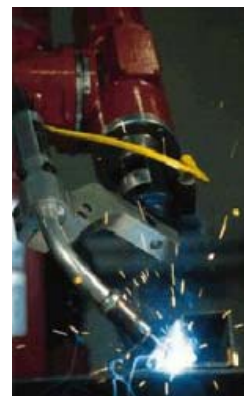
Figure 2 (a) Gas welding (b) Schematic of Arc welding (c) Arc welding is easier to automate using Robots (why?)
